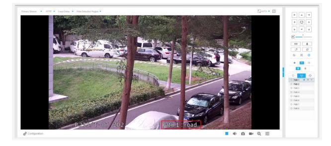
Step2: Use the PTZ control buttons to move the lens to the interested position;
