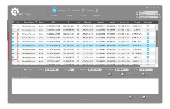
**Step4:** If the selected camera shows "Inactive" in the status bar, click "Activate" to set the password when using it for the first time. You can also set the security questions when activating the camera in case that you forget the password (You can reset the password by answering three security questions correctly). Click 'Save' and it will show that the activation was successful.
