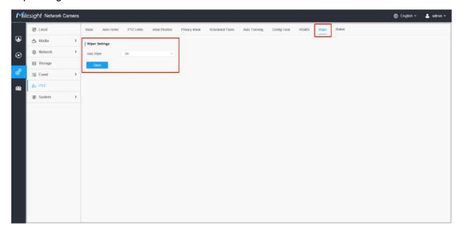
In the live view interface, it also supports manually enabling the wiper to wipe twice by clicking the wiper button or directly calling the preset 53.
