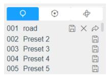
Note: The following presets are predefined with special commands. You can only call them but can't configure them. For example, preset 037 is the "Self Check". If you call the preset number 037, the PTZ camera will start self check function at once.
