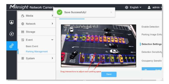
**Step 6:** After the configuration, the occupied parking spaces in the detection area will be covered with red to provide a more intuitive interface. And the parking information containing total number, occupied number and available number will be displayed on the interface.
