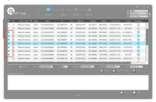
**Step4:** If the selected camera shows "Inactive" in the status bar, click "Activate" to set the password when using it for the first time. You can also set the security questions when activating the camera in case that you forget the password (You can reset the password by answering three security questions correctly). Click 'Save' and it will show that the activation was successful.
