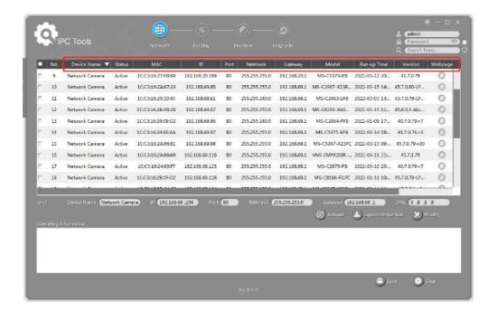
**Step3:** Select a camera or multiple cameras according to the MAC addresses;
