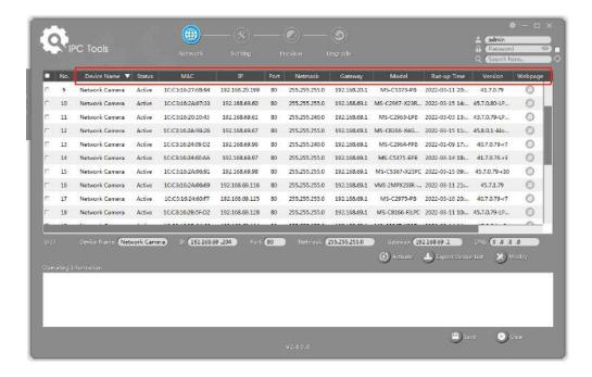
**Step3:** Select a camera or multiple cameras according to the MAC addresses; Select single camera:
