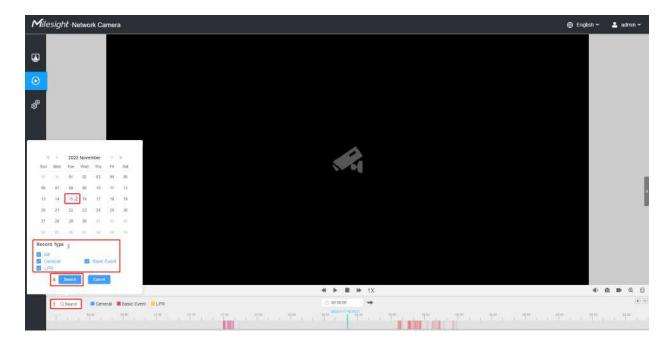
**Step2:** The timeline displays the video files for the day and show different colors according to selected record type. Drag the progress bar with the mouse to locate the exact playback point as needed.
