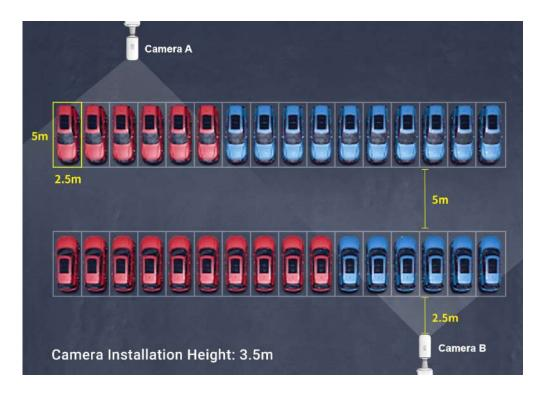
**Note:** The red car area is detected by Camera A, and the blue car area is detected by Camera B.
