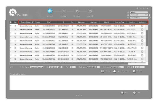
**Step3:** Select a camera or multiple cameras according to the MAC addresses;
