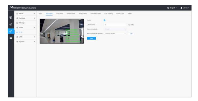
Auto Home allows the PTZ camera to return to a predefined Home Position automatically after a period of latency time. Check the checkbox to enable the Auto Home mode.
